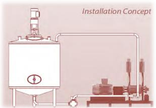
ROTOCAV equipment can be installed in new plants or it can be integrated as a booster in existing plants, requiring few modifications.
